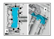
Close valve on gas tank No. 3 in direction of arrow using handwheel -T50026-(ŠKODA special tool) or pliers.
