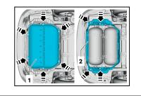
Close valve on gas tank No. 2 in direction of arrow using handwheel -T50026-(ŠKODA special tool) or pliers.
